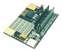
A charger can be connected to the **CHARGE** terminal. Charging current must be less than 1A. If you need to charge
